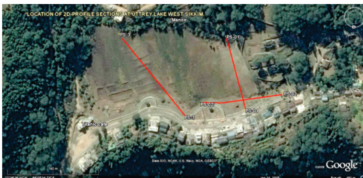
Fig. 2 location map of the Uttarey Lake showing the electrical resistivity Profiling.
